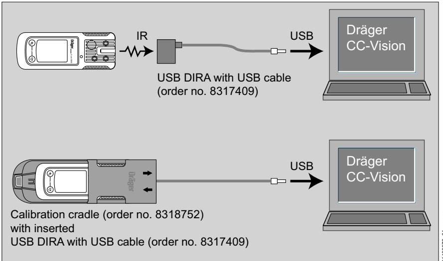
The installed PC software Dräger CC Vision is used for configuration.
